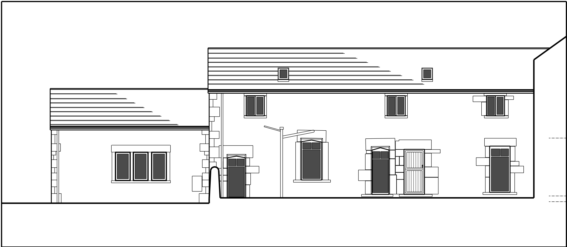
Dwelling North Elevation - Existing
