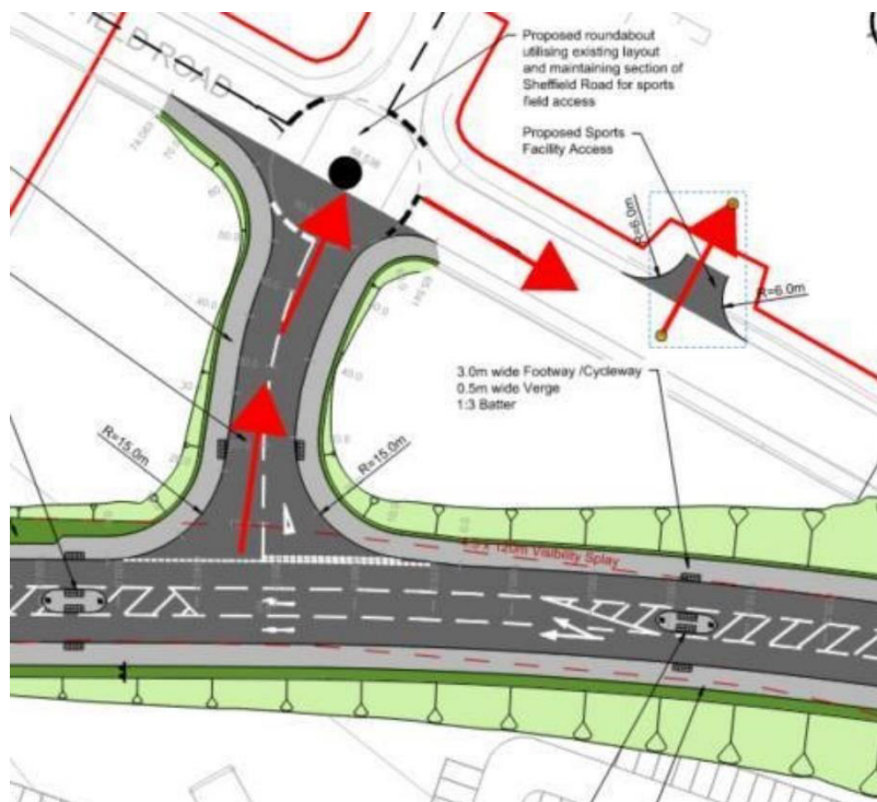
Figure 3 Route for Moving Material
